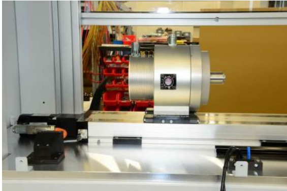
The linear axis can be positioned exactly using an AKD & AKM one-cable package (incl. control unit). The KBM Kit motor which is responsible for synchronization of the tubes fed through sits on top of this.
